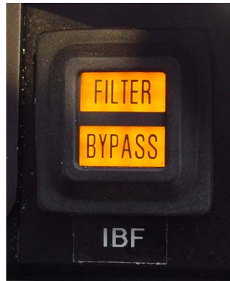
Picture 6: -103 Cockpit switch/indicator
