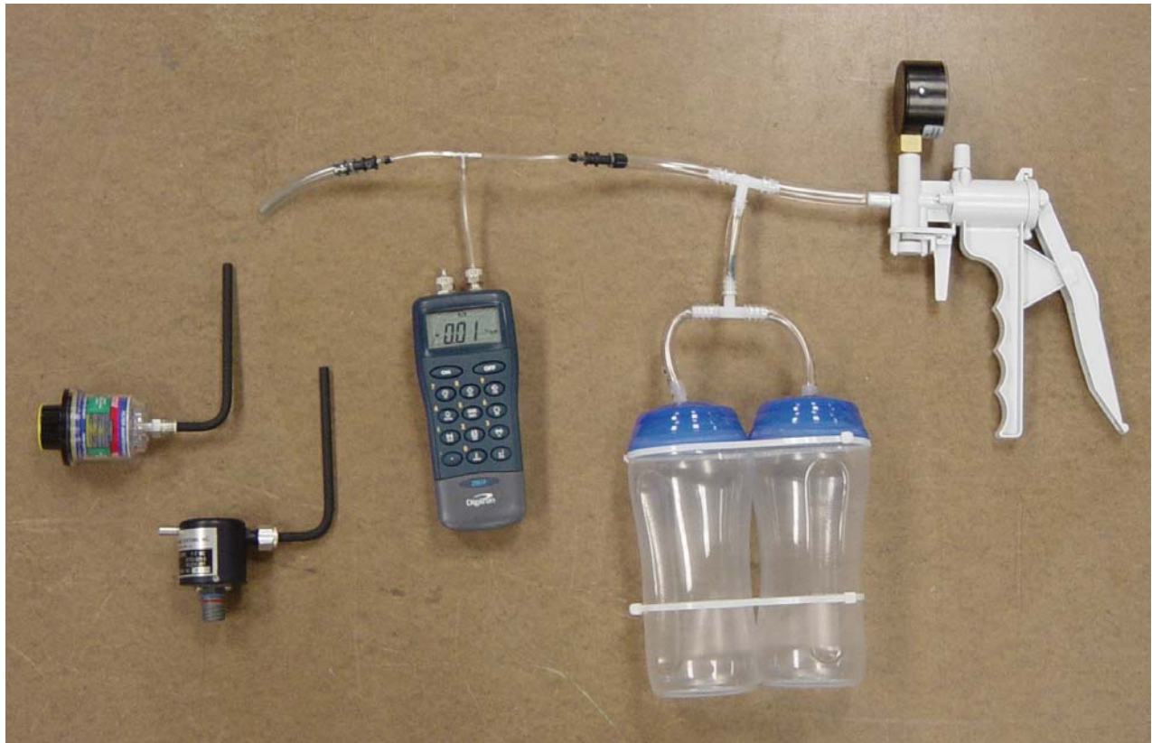
Picture 7: Test Setup with Manometer
